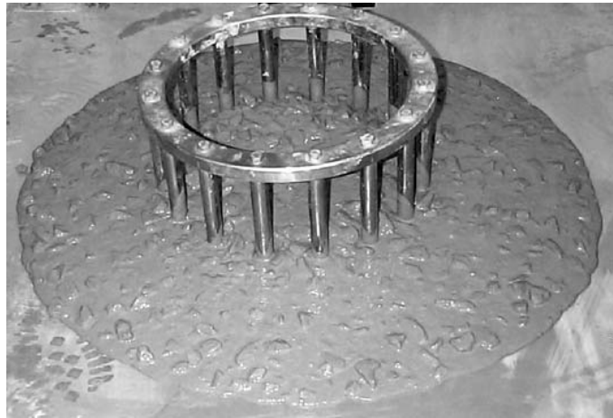
Figure 2.5 – J-Ring flow after lifting the mold (ASTM C1621 2014).
